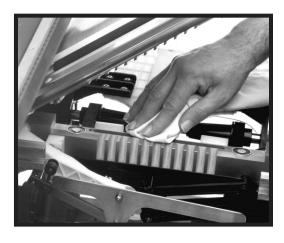
Remove any debris from the comb. Clean the film gripper on the center clamp with a soft cloth dampened with isopropyl alcohol (recommended) or hot water. Wipe the surfaces dry when done cleaning. (This must be dry before using the machine.)
