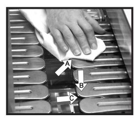
Clean the pressure rollers with a soft cloth dampened with hot water. Remove any debris from the rollers.
