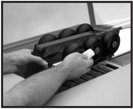
Raise the lifter by pulling it up. Clean the lifter supports with a soft cloth dampened with hot water. Remove any debris from the supports.
