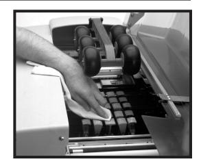
Clean the Infeed Belts and the Infeed Door with a soft cloth dampened with hot water. Wipe the belts and rollers to remove any grease or debris.
