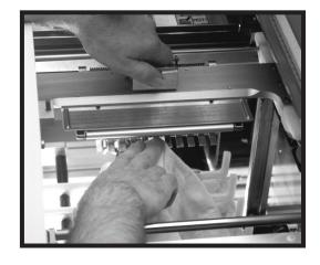
Clean the roller on the center clamp with a soft cloth dampened with hot water. Remove any debris from the roller.
