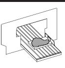
The trays must be in line against the Start Switch for proper wrapping.
