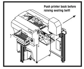
Raise the sealing belt using the handle for access to the distributor, film clamp, and folders below it. **Caution! The belt may be hot.** Clean the film folders, distributor, and curved rollers with a soft cloth dampened with hot water.
