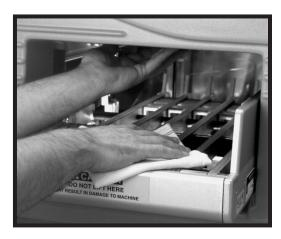
If your system is a SOLO® XL Combo, remove the scale risers, then the scale platter by lifting the platter up and out. Clean both daily using hot water, soap, and a brush to clean the slots.
