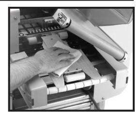
While the Sealing Belt is raised, clean the distributor film clamp with a soft cloth dampened with hot water. When lowering the sealing belt, hold the handle and lower it gently to avoid alignment problems.
